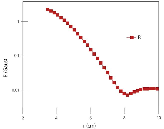
**Figure 3:** Radial profile of the  $B_z$  magnetic field strength measured with the single loop
