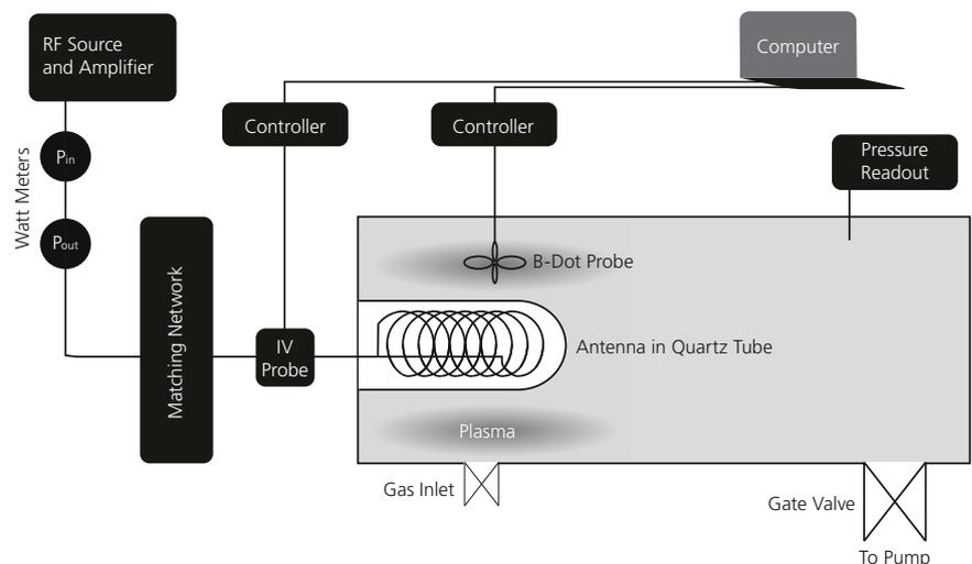
Figure 1: Experimental setup
