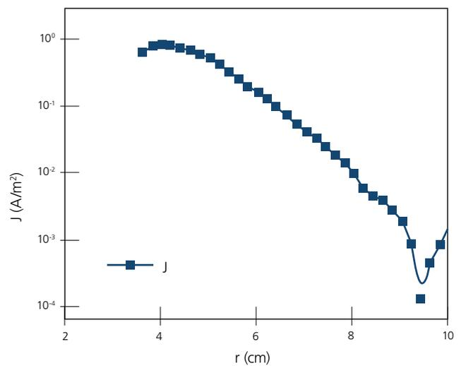
Figure 6: Radial profile of the calculated azimuthal current density
