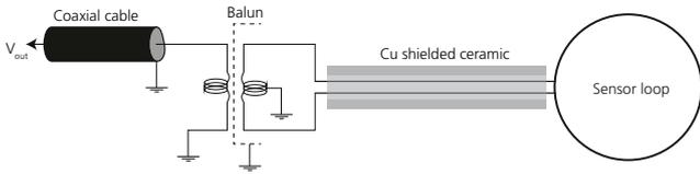
**Figure 2:** Schematic of the single loop B-Dot probe element
