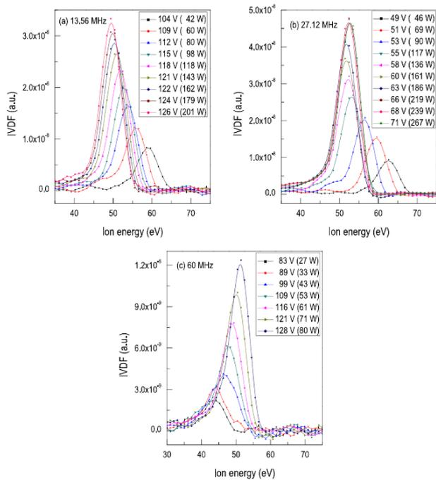
Figure 6. Variation of maximum ion energy with discharge voltage at different pressures for the (a) 13.56 MHz, (b) 27.12 MHz and (c) 60 MHz driven magnetron sputtering discharge.
