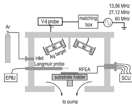
Figure 1. Schematic of the magnetron sputtering discharge setup.
