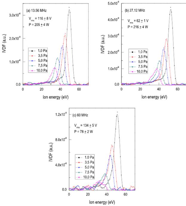
Figure 2. Variation of IVDFs with pressure for the (a) 13.56 MHz, (b) 27.12 MHz and (c) 60 MHz driven magnetron sputtering discharge at discharge voltages of  $V_{rms}=116\pm 8V$ ,  $V_{rms}=62\pm 1V$  and  $V_{rms}=134\pm 5V$ , respectively.
