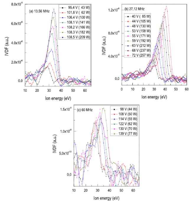
Figure 5. Variation of IVDFs with discharge voltage (or sputtering power) at the pressure of 10.0 Pa for the (a) 13.56 MHz, (b) 27.12 MHz, and (c) 60 MHz.
