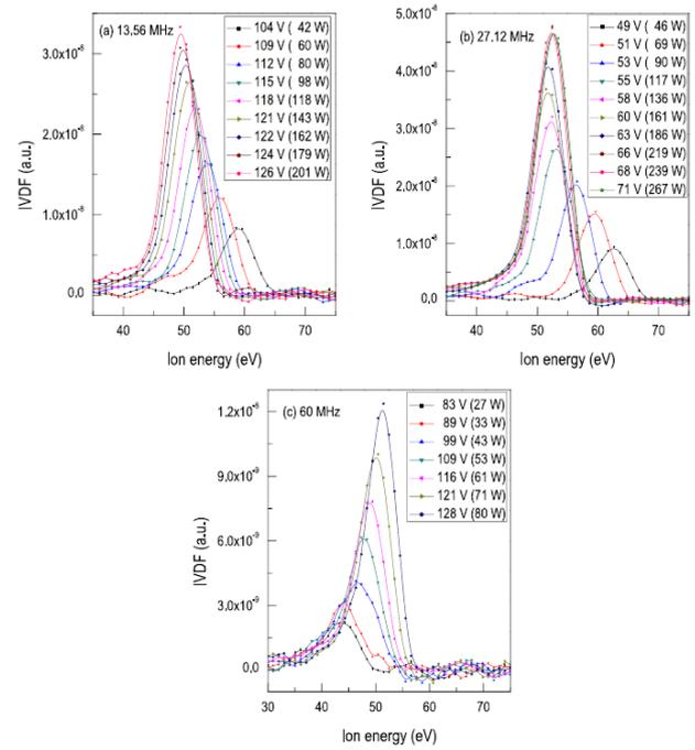
Figure 4. Variation of IVDFs with discharge voltage (or sputtering power) at the pressure of 1.0 Pa for the (a) 13.56 MHz, (b) 27.12 MHz, and (c) 60 MHz driven magnetron sputtering discharge.
