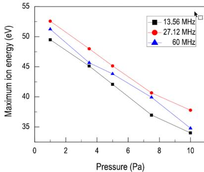
Figure 3. Variation of maximum ion energy with pressure for the 13.56 MHz, 27.12 MHz and 60 MHz driven magnetron sputtering discharge at discharge voltages of  $V_{rms}=116\pm 8V$ ,  $V_{rms}=62\pm 1V$  and  $V_{rms}=134\pm 5V$ .
