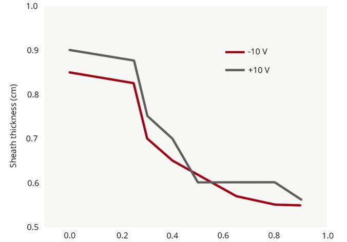
Figure 4. Sheath thickness vs negative ion concentration in the diffused section for  $V_{plate} = \pm 10V$ .
