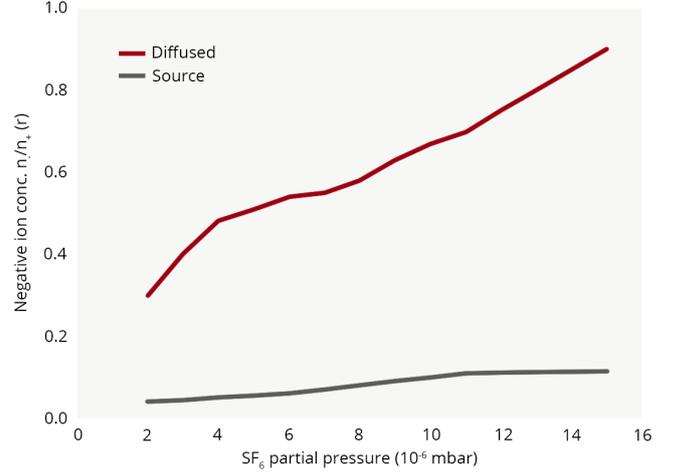
Figure 3. Comparison of the negative ion concentration ( $r$ ) vs  $SF_6$  partial pressure in the Source ( $F$ ) and diffused ( $SF_6$ ) sections.
