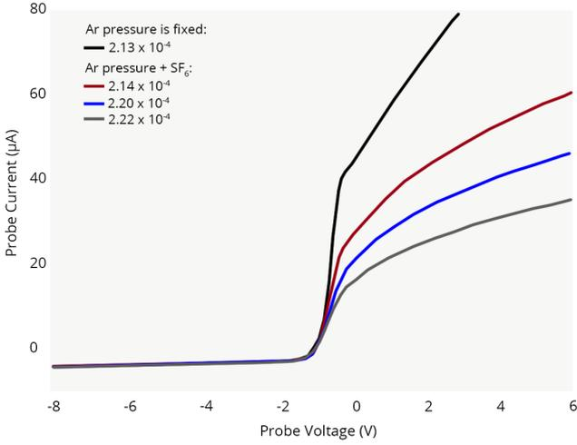
Figure 2. Comparisons of Langmuir probe I-V characteristics for different  $SF_6$  concentrations.
