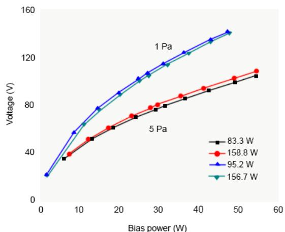
Figure 7. Discharge voltage on the substrate versus bias power for different sputtering power at 5 Pa and 1 Pa.
