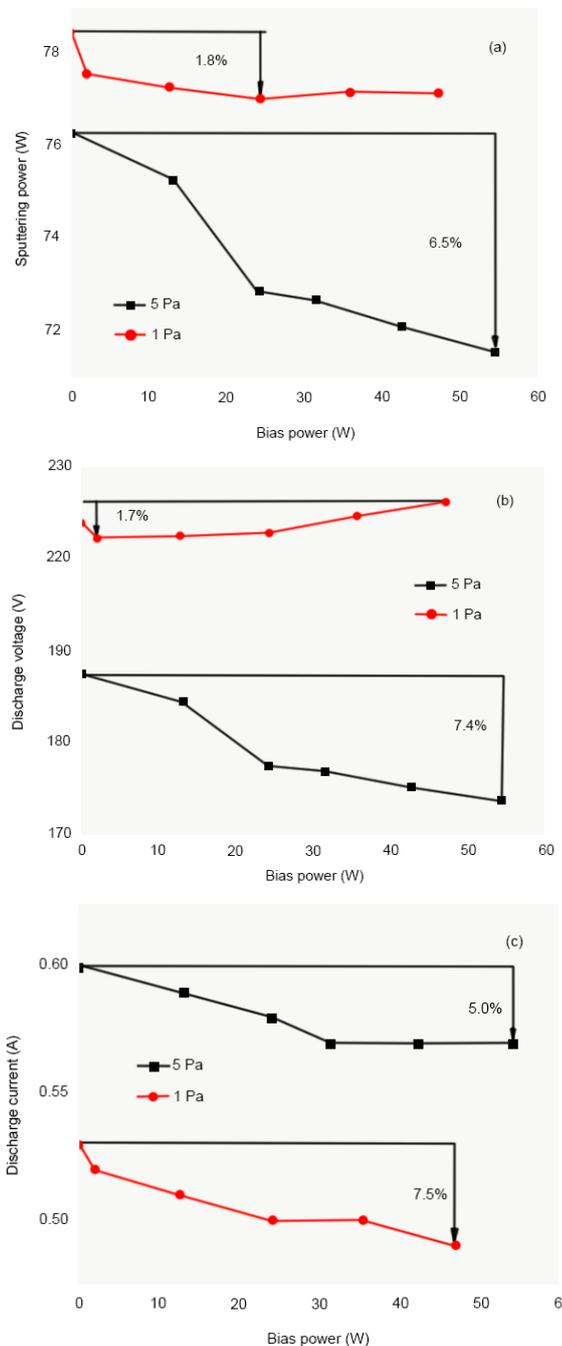
Figure 3. Effect of the bias power on the (a) sputtering power, (b) discharge power and (c) discharge current at 5 Pa and 1 Pa.
