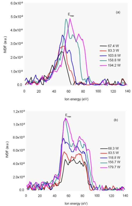
Figure 4. Variation of IVDFs with sputtering power (without bias) at (a) 5 Pa and (b) 1 Pa.
