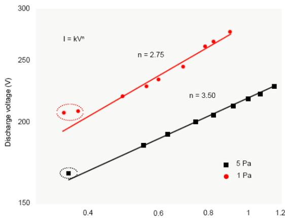
Figure 2. Log(I)-Log(V) curves of 2 MHz magnetron sputtering at 5 Pa and 1 Pa.
